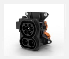
Vehicle charging inlet for charging with direct current (DC), compatible with type 2 CCS vehicle charging connectors (EVSE), for installation in electric vehicles (EV).
